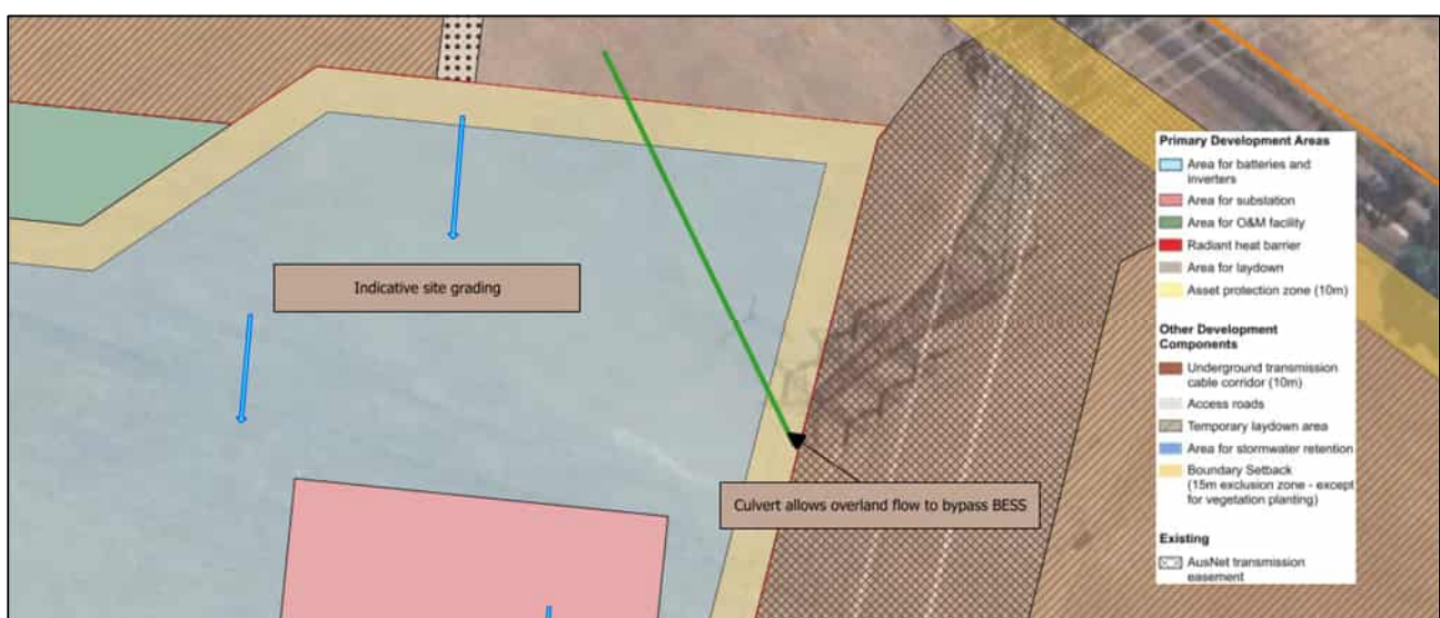
Figure 10: Concept plan of external overland flow path culvert
